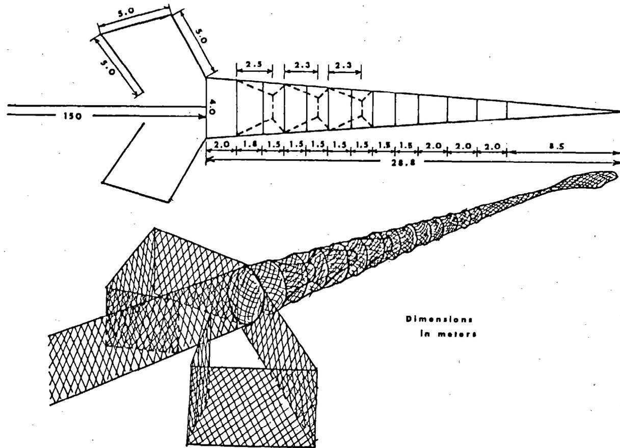
Figure 4.- Diagram of a traditional fishing device used for capturing saffron cod in Pacific waters of the U.S.S.R. (from Andreev 1962).
