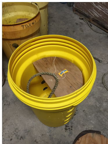
Poly Drum Station with two snap traps (Victor and T-Rex) and an indicator bait.
