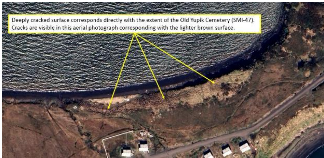
Figure 22. High density of deep cracks resulting from earth pulling away to the ocean.
