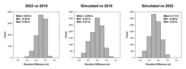
**Figure 4.** Assessing the accuracy of differencing the three digital terrain models (DTMs) used in our assessments of elevation change. The difference in elevation values was extracted from a 30 m x 30 m area that appeared to have remained stable and undisturbed between 2016 and 2022. Left, 2022 DTM versus 2016 DTM; middle, simulated DTM versus 2016 DTM; right, simulated DTM versus 2022 DTM.
