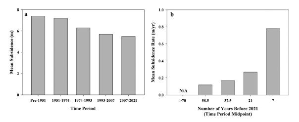
**Figure 10.** Estimated mean terrain subsidence magnitude and rates based on the difference in elevation between the simulated DTM and the drone system DTM relative to the time periods of thermokarst lake expansion determined with the remote sensing time series imagery. As shown here, thermokarst processes led to rapid rates of subsidence in the first decade following disturbance but diminished over time as the lake deepened.
